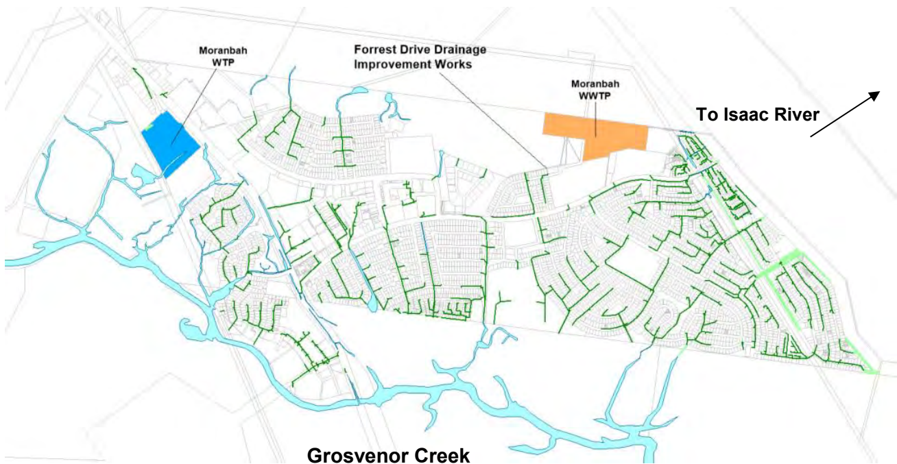
Figure 8: Moranbah Stormwater Network with formal drainage infrastructure (dark green), open swale drains (light green) and surface waters (blue)
