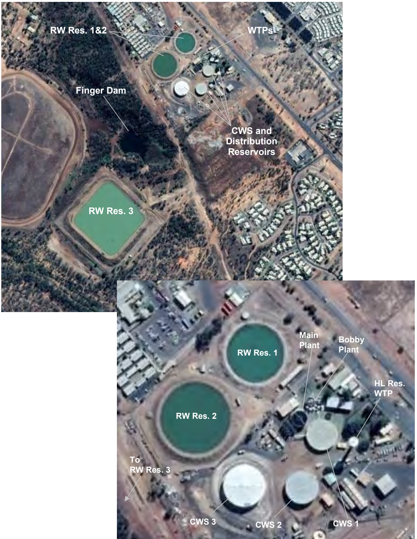
Figure 3: Moranbah Water Treatment Plant Layout
